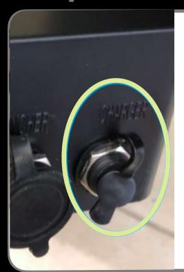
Remove battery drawer. Open cover of charger connector.
