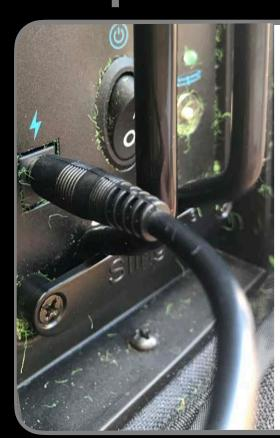
Plug power charger into the charger connector.
