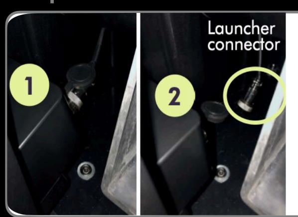
Disconnect the battery wire from the launcher connector.
